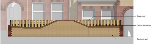
③ Refuse Storage Elevation 2 1:50
