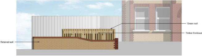
② Refuse Storage Elevation 1 1:50
