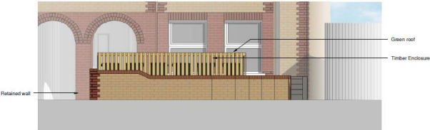
④ Refuse Storage Elevation 3 1:50
